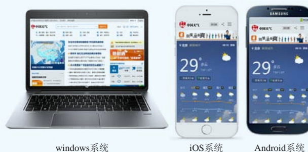
图1 应用响应式布局的网站示意图 Fig. 1 Application of response layout on website
