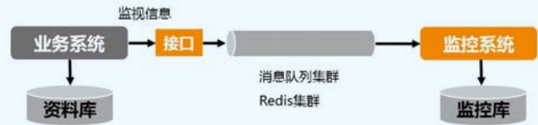
图3 “松耦合”的技术架构 Fig. 3 Loosely coupled technical architecture
