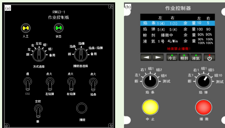
图4 作业控制器界面布局对比 (a) 东北新舟60增雨飞机；(b) 西北新舟60增雨飞机 Fig. 4 Comparisons of seeding control interface (a) MA60 of Northeast project, (b) MA60 of Northwest project
