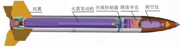
图7 探空火箭组成及内部结构 Fig. 7 Composition and internal structure of rocket sounding
