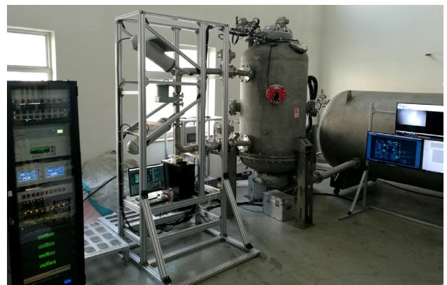
图3 中国气象科学研究院绝热膨胀云雾舱系统 Fig. 3 The adiabatic expansion fog chamber system of Chinese Academy of Meteorological Sciences
